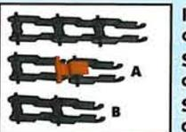
If you need to take up slack in black Chain Links, (A) substitute a small gold Splice piece, or (B) remove a black Link.
