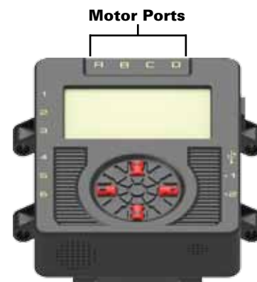
Figure 6: K’NEX Robotics Control Box - Front Face
